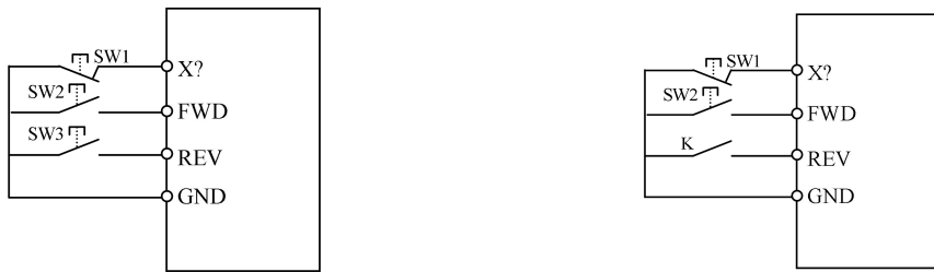
a) Three-wire control mode 1 wiring diagram b) Three-wire control mode 2 wiring diagram
